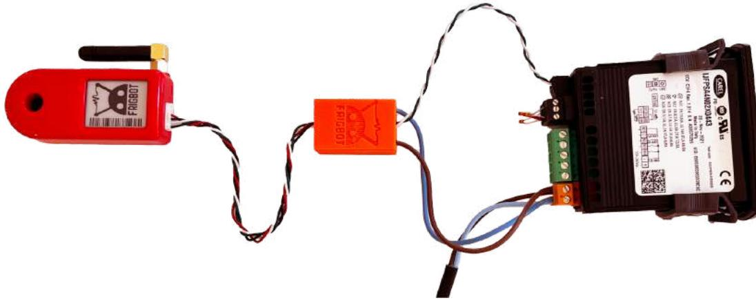
Frigbot® was made to work with Carel®. The installation and configuration of your new Frigbot are really easy. If you're a licensed tradesperson you can also install the additional current sensor that allows you to read the power usage and set alerts for when something is going wrong, more about this later.
