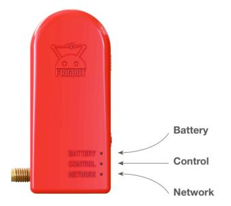
**BATTERY** is RED colour LED indicator Solid RED = battery full Slow Blink = battery LOW (charging)
