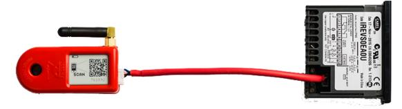
Frigbot® was made to work with Carel®. The installation and configuration of your new Frigbot are really easy. If you're a licenced tradesperson you can also install the additional current sensor that allows you to read the power usage and set alerts for when something is going wrong, more about this later.
